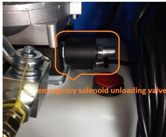
2. Take off the protective cap of the valve and see red the valve core.
